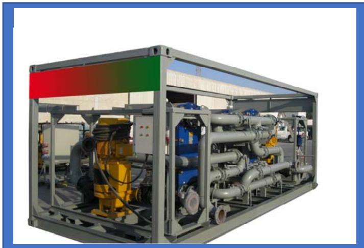
Heat Exchanger Skid
