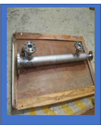
Level Transmitter Chambers
